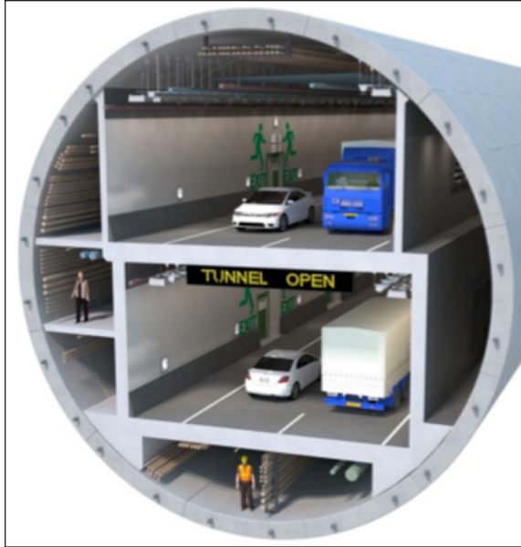
Figure 1. SR 99 bored tunnel cross section—design concept
